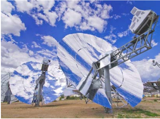
A Stirling Engine and a point focal parabolic dish. Photo: Randy Montoya at Sandia National Laboratories (used by permission).
